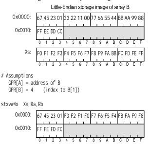
Figure 128.Process to store unaligned quadword to Little-Endian storage Store VSX Vector Word\*4 Indexed
