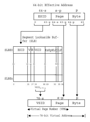
Figure 27. Translation of 64-bit effective address to 78 bit virtual address
