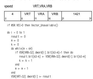
For each integer value i from 0 to 1, do the following. Starting from the right, for each bit in doubleword element i of VSR[VRB+32] that is equal to 1, place the contents of the corresponding bit in doubleword element i of VSR[VRA+32] into the rightmost unoccupied bit of doubleword element i of VSR[VRT+32]. Any bits in doubleword element i of VSR[VRT+32] to the left of the most-significant bit copied are set to 0.
