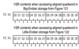
Figure 123.Vector-Scalar Register contents for aligned quadword Load or Store VSX Vector
