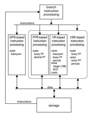
Figure 1. Logical processing model
