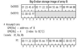
Figure 125.Process to load unaligned quadword from Big-Endian storage using Load VSX Vector Word\*4 Indexed
