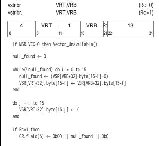
From right-to-left, the contents of each byte element of VSR[VRB+32] are placed into the corresponding byte element in VSR[VRT+32]. If a byte element in VSR[VRB+32] is found to contain 0, the corresponding byte element and all byte elements to the left of that byte element in VSR[VRT+32] are set to 0.
