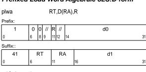
$$\label{eq:continuous} \begin{split} &\text{if "Iwa" then} \\ &\text{EA} \leftarrow (\text{RA}|0) + \text{EXTS64}(\text{DS}||0\text{b00}) \\ &\text{if "pIwa" & R=0 then} \\ &\text{EA} \leftarrow (\text{RA}|0) + \text{EXTS64}(\text{d0}||\text{d1}) \\ &\text{if "pIwa" & R=1 then} \\ &\text{EA} \leftarrow \text{CIA} + \text{EXTS64}(\text{d0}||\text{d1}) \end{split}$$
