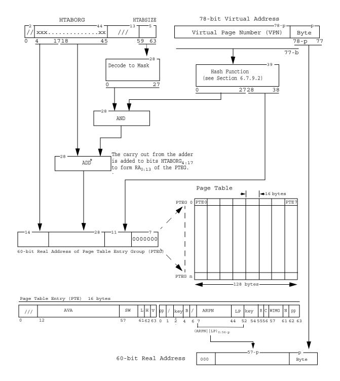
Figure 31. Translation of 78-bit virtual address to 60-bit real address
