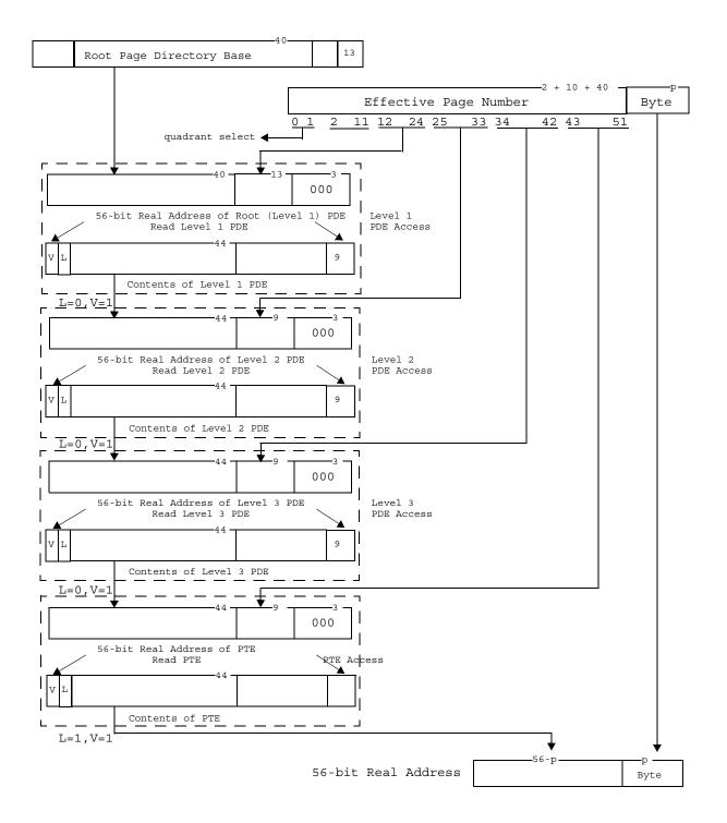
Figure 34. Four level Radix Tree walk translating a 52b EA with NLS=13 in the root PDE and NLS=9 in the other PDEs.
