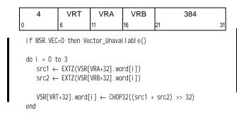
For each integer value i  $% \left( 1\right) =1$  from 0 to 3, do the following. The unsigned integer value in word element i in VSR[VRA+32] is added to the unsigned integer value in word element i in VSR[VRB+32]. The carry out of the 32-bit sum is zero-extended to 32 bits and placed into word element i of VSR[VRT+32].
