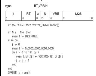
Starting with bit 0, the contents of every  $N^{th}$  bit of VSR[VRB+32] are concatenated and placed into GPR[RT].
