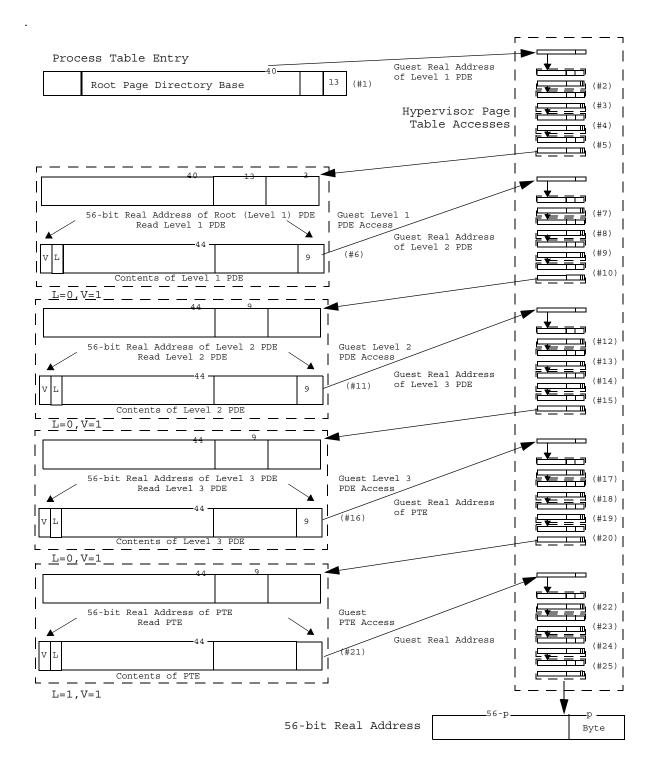
Figure 37. Radix on Radix Page Table search for a 52-bit EA depicting memory reads 1-24 numbered in sequence
