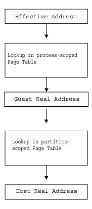
Figure 26. Address translation overview, Radix on Radix
