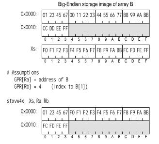
Figure 127.Process to store unaligned quadword to Big-Endian storage using Store VSX Vector Word\*4 Indexed
