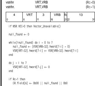
From right-to-left, the contents of each halfword element of VSR[VRB+32] are placed into the corresponding halfword element in VSR[VRT+32]. If a halfword element in VSR[VRB+32] is found to contain 0, the corresponding halfword element and all halfword elements to the left of that halfword element in VSR[VRT+32] are set to 0.
